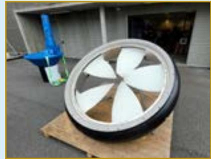
Framo's SR2000 flow generator is used to pump large volumes of water vertically for salmon cages which use lice skirts. The innovative design features a permanent magnetic motor and water-lubricated bearings.
