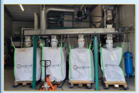
This BioRetur facility receives sludge from the salmon hatchery next door and stabilizes it for use in fertilizer products.
