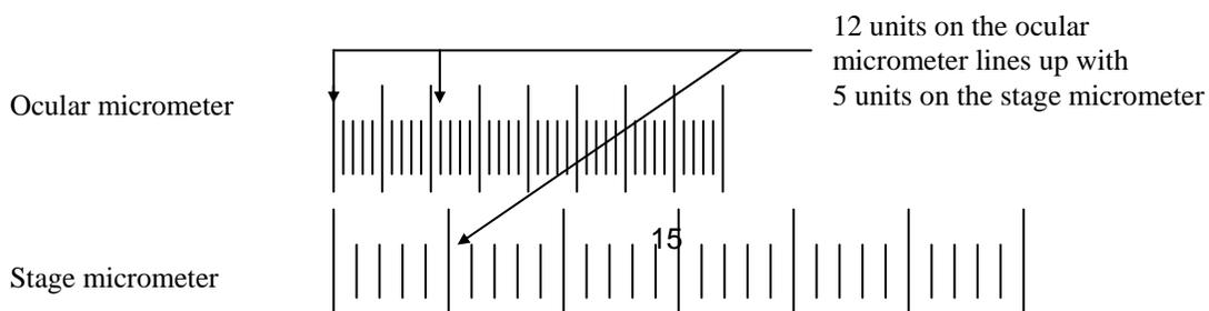
4. Divide the number of ocular micrometer lines by the number of stage micrometer lines (a).
