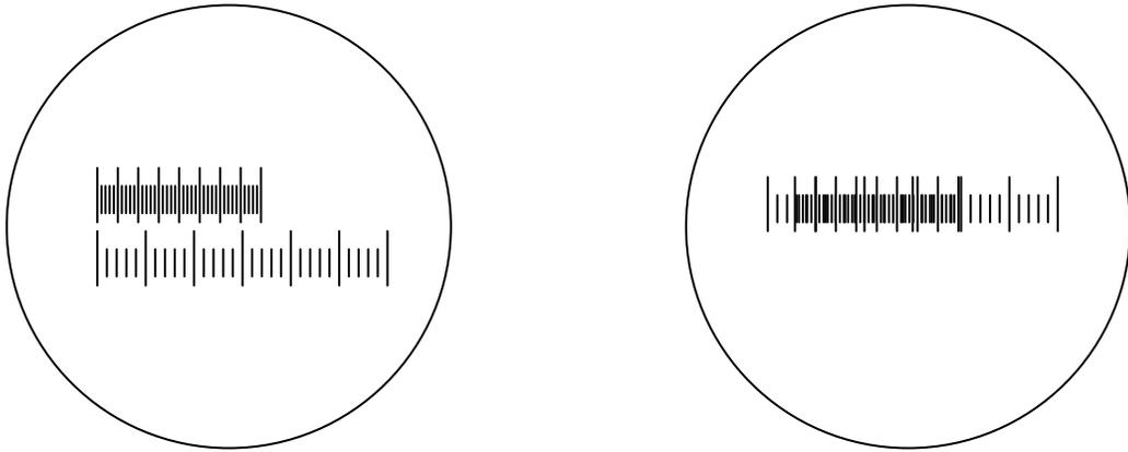
2. Move the stage micrometer until one line of the stage micrometer coincides with a line of the ocular micrometer (a). Then look for another line along the stage micrometer that coincides with a line on the ocular micrometer (b).
