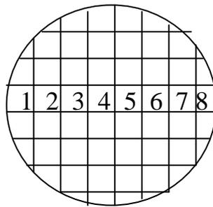
In this example, 8 squares fit across the field of view, so the diameter is 8 mm or 8000  $\mu\text{m}$ . To determine the size of individual larvae, estimate how many of these will fit across the field of view if they were lined up end to end. If approximately 32 could fit across, then each larvae is  $8000 \div 32 = 250 \mu\text{m}$ . Note that each time you change to a different power of magnification, you must determine the field of view.
